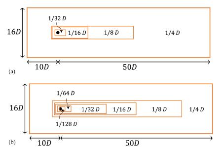
FIG. 4. Meshing in simulation and the location of refinement levels. The computational domain is (x, y, z) = ([-10, 50], [-8, 8], [-8, 8])D and the results in ([1.5, 15], [-2, 2], [-2, 2])D was used. (a) Mesh for Re = [200, 300, 500] has four refinement levels:  $2^{-[2\cdots 5]}D$  (b) Mesh for Re = 1000 has six refinement levels:  $2^{-[2\cdots 7]}D$ .
