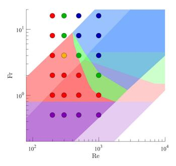
FIG. 5. A regime diagram for stratified sphere wakes. The final result in colored dots combines experiments from CH93 (lighter colors) and LI92 (darker colors) with combined laboratory and numerical experiment. The five identified regimes are labeled and color coded as: Vortex street (VS, purple), Symmetric nonoscillatory (SN, red), Asymmetric nonoscillatory (AN, yellow), Planar oscillatory (PO, green), and Spiral mode (SP, blue).
