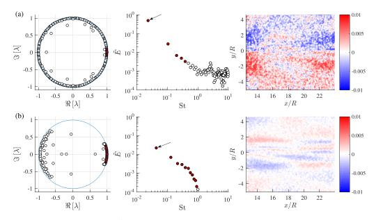
FIG. 13. Ritz values  $\lambda$  (left),  $\tilde{E}$  versus St (center), v(x, y, z = 0) of a dominant oscillatory mode (indicated by an arrow) for the Re = 300, Fr = 2 case computed from (a) standard DMD ( $E_r = 100\%$  of  $\tilde{E}$ ) and (b) TDMD ( $E_r = 91.6\%$ ). Modes colored in red are energetic modes selected from Sec. III C 1.
