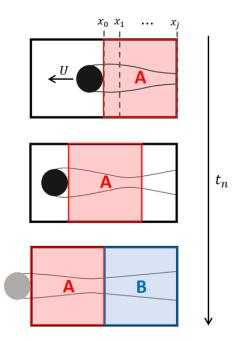
FIG. 3. Temporal data reconfiguration where the colored box A is moving in reference to the sphere. Dashed lines indicate column vectors of velocity field within the box A.
