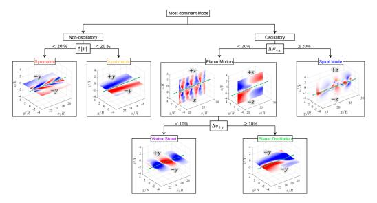
FIG. 10. A flow chart of the wake classifier with two, 2D-center-plane flow fields as input. Two dominant DMD modes of each center plane are evaluated where the mode for the vertical center plane is selected based on  $St_w$  closest to  $St_v$ . The nonoscillatory branch uses the mode from the horizontal center plane, while the oscillatory branch uses the vertical centerplane for the first step, and horizontal centerplane for the second step. Green dotted line represents the wake centerline.
