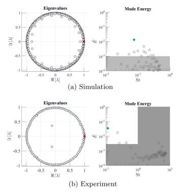
FIG. 7. The plots on the left show the real and imaginary parts of  $\lambda$ , and on the right  $\tilde{E}(St)$  is shown for each mode of the case Re = 500 and Fr = 4. The dark red corresponds to the mean mode. The green dot is the most dominant mode selected to be evaluated in Fig. 8. The grey area is considered noise, set below  $\tilde{E}$  threshold and above St threshold. (a) Simulation, (b) Experiment.
