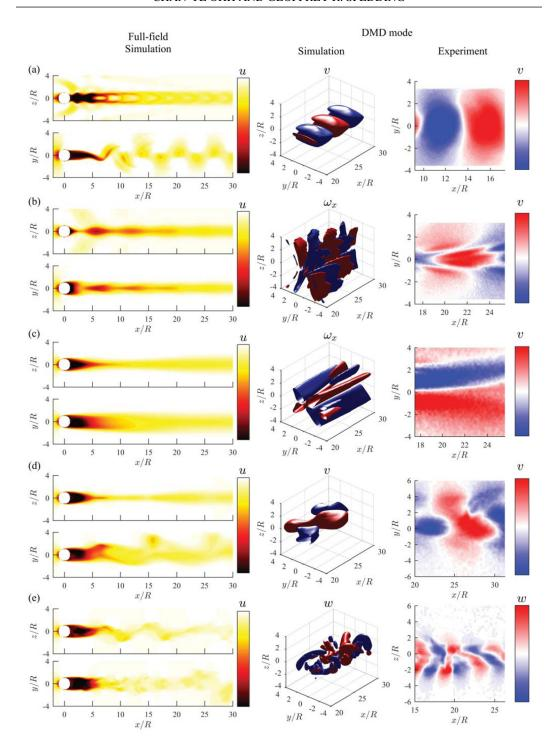
FIG. 6. A snapshot of the flow field u in vertical and horizontal centerplane (left) and a dominant DMD mode of simulation in 3D (middle) and experiment in 2D center plane (right) illustrating various regimes observed: (a) R10F0.5 Vortex Street (R2F0.5 for the experiment), (b) R5F1 Symmetric nonoscillatory, (c) R3F4 Asymmetric Nonoscillatory, (d) R3F8 planar oscillatory (e) R10F8 spiral mode. The isolevel of the middle 3D plot is 30% of the maximum velocity component.
