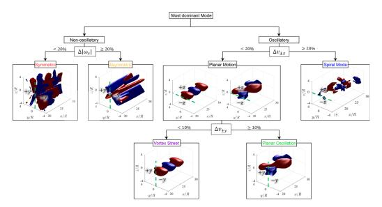
FIG. 8. A flow chart of the wake classifier with 3D DMD input. The selected DMD mode from Sec. III C 1 is sorted into five regimes in the nonoscillatory branch (left) and oscillatory branch (right) based on the symmetry of the cross-stream velocities in that mode.
