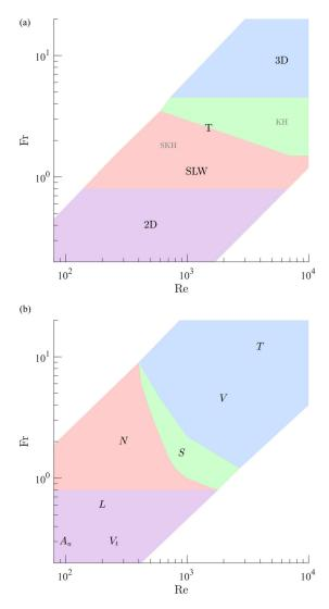
FIG. 1. Regime diagrams from CH93 (a) and LI92 (b). The four main regimes differentiated in (a) are 2D, quasi-2D; SLW, strong lee wave; T, transition (SKH, without K-H instability; KH, with K-H instability); and 3D, three-dimensional. In (b), LI92 distinguished six main regimes:  $A_u$ , unsteady, attached 2D vortices;  $V_t$ , 2D vortex shedding; L, lee-wave instability; N, nonaxisymmetric attached vortex; S, symmetric vortex shedding; V, nonsymmetric vortex shedding; and T, turbulent wake.
